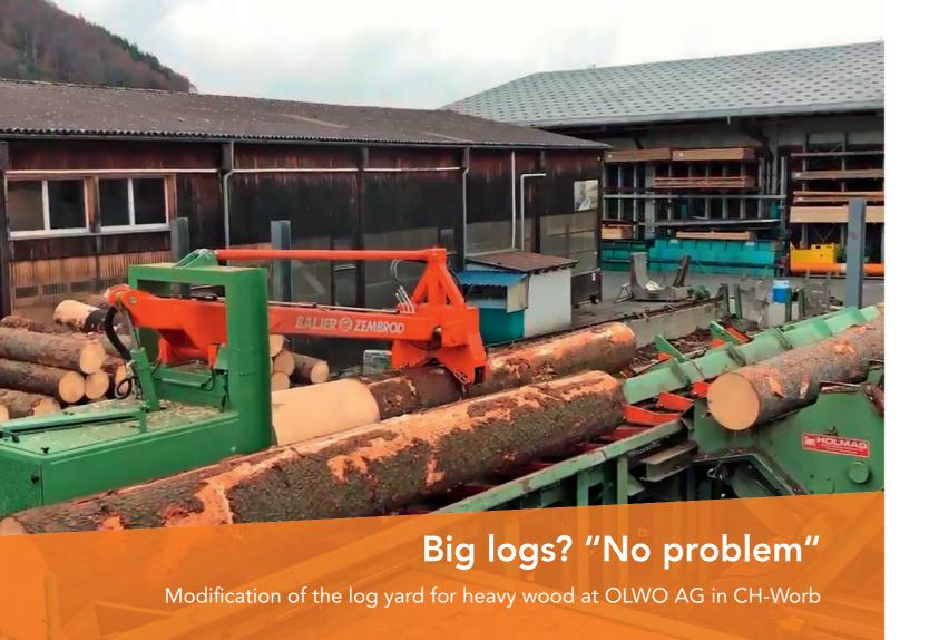
A laser measuring has been integrated in the existing cross transfer in front of the cutting conveyor. The operator cuts the logs on the crosscut conveyor based on the measured log length and a visual assessment.
