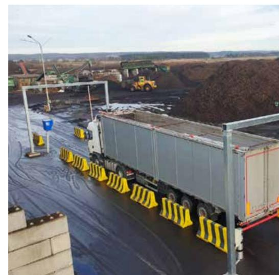
In addition to log measurement, the JORO-volume truck scanner is the second business line of JE. This measurement technology records the load volume of trucks and is also used in the wood processing industry.
