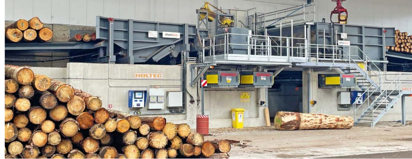
"Due to the strict task separation and implementation with two lines, it was possible to tailor each line to the requirement profile in the best possible way", explains Bannert. "High cycle rates and fast processes were decisive for the line with small diameter logs. A robust, heavy design of the system components was required for the line with big diameter logs."
