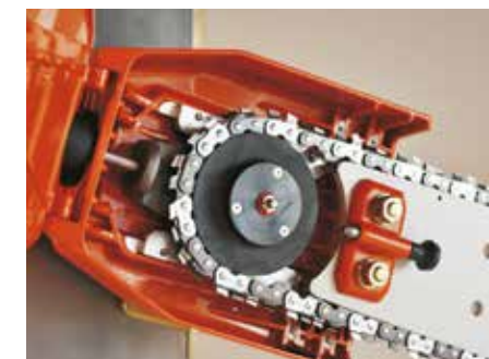
Fast chain replacement without additional tools
