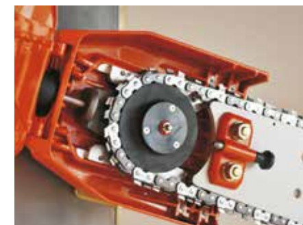
Fast chain replacement without additional tools
