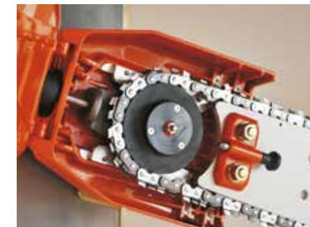
Fast chain replacement without additional tools
