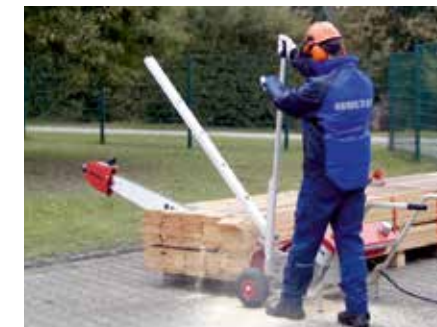
Easy handling and low power requirement during cutting process. Pneumatic tires and 3-fold machine supports guarantee exact positioning and an angularly cut - under nearly all conditions. Available with pneumatic tires or solid tires.
