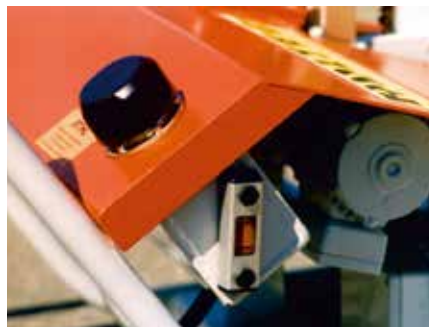
Separate drive for lubrication oil pump - this guarantees a constant lubrication under all conditions. Lubricant tank sufficient for approx. 4 h operation time.
