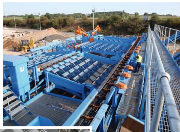
View to step feeders and butt reducers at James Jones, UK
