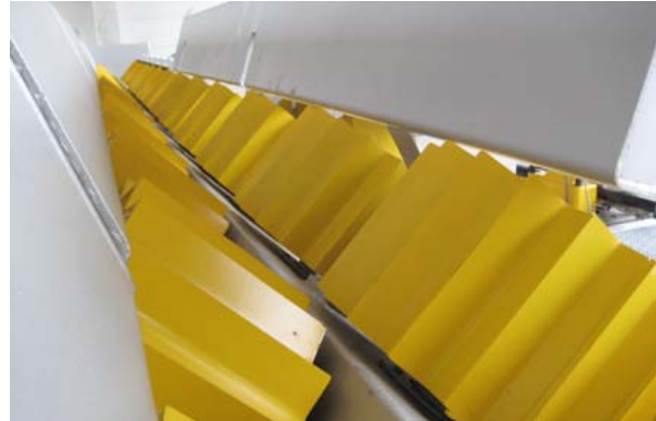
The v-rollerway – pairs of rollers at right angles to each other that set new standards in the field of log acceleration
