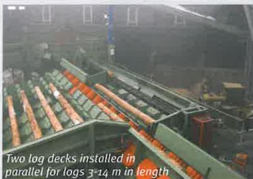
range. Smaller bar lengths are separately transferred to the longitudinal conveyor. For longer bars, the two feeding systems work synchronically. The proven rollerway from Holtec is installed at van Roje as well. All bars are fed to this rollerway. The rectangular aligned pairs of rollers assure a safe acceleration and avoid a lateral sliding of the bars with diameters from 100-700 mm. The v-rollerway with 18 pairs of rollers is the
