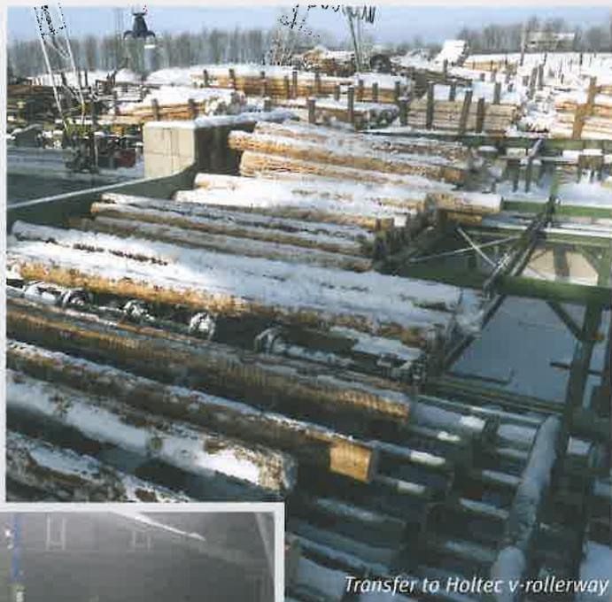
longest of its type. The logs are sawn at several preselected speeds, depending on the sawing pattern. The v-rollerway with separately controlled drives in combination with a dynamic gap optimisation Holtec GapControl provides for a precise and minimal gap between each log. All components are designed for an
