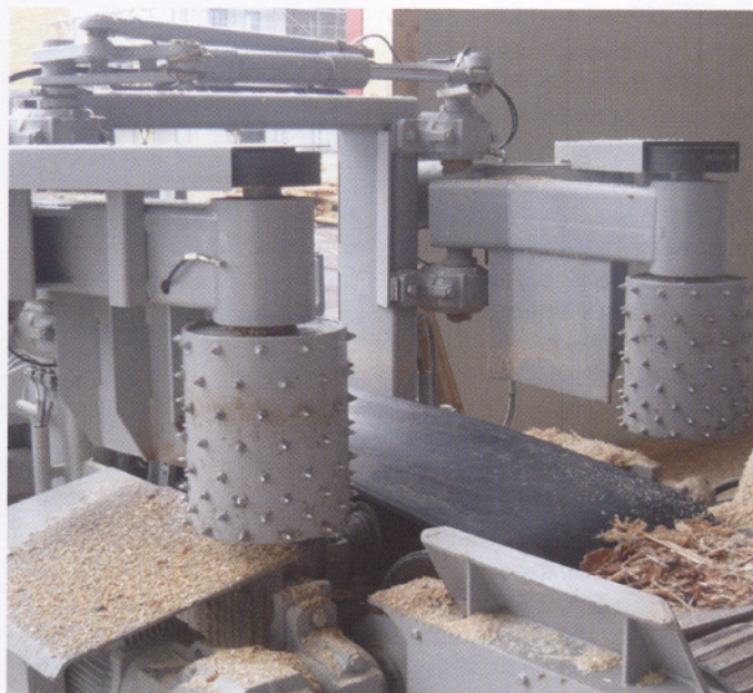
The aligning system leading to the Holtec cross-cut saw
