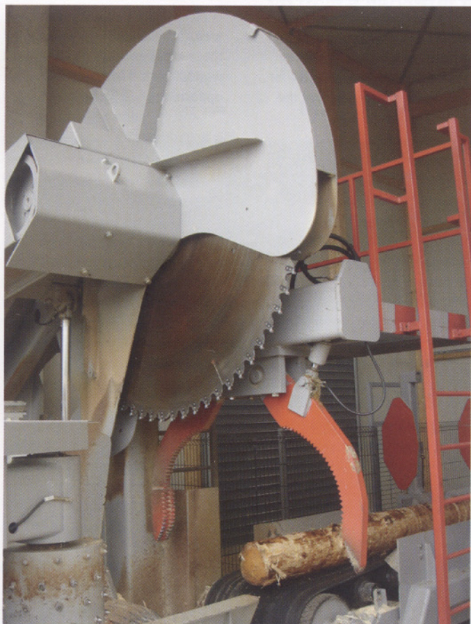
The recently installed Holtec cross-cut saw
